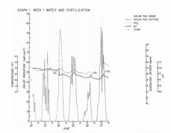
GRAPH I. This figure represents the first week of monitoring Solar-Algae Pond AI9 inside the Cape Cod Ark. Dissolved oxygen is in parts per million and solar radiation in milliwatts/cm.<sup>2</sup> The pond temperature was measured once daily while the others were measured continuously. The chart recorder ran somewhat erratically, creating the discrepancy between real time and expected sunlight intensities.
